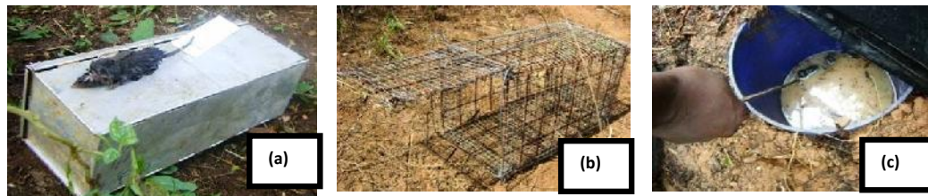
Figure 2: (a) Sherman live trap, (b) live wire cage or spring door trap and (c) bucket used for pitfall trap
